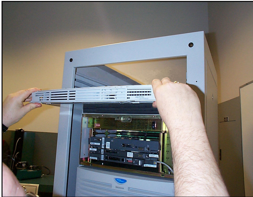
Figure 57 Rack-mounting the ISP1100 Signaling Server
