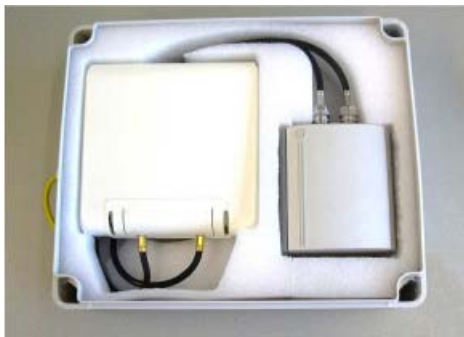
Figure 84: 4720 DAP and directional antenna in their positions
