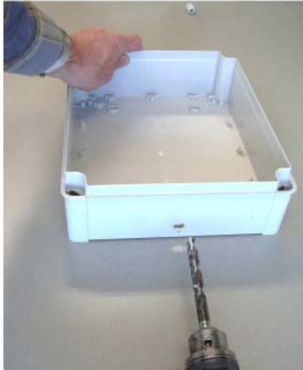
Figure 72: Drilling the hole (12 mm)
