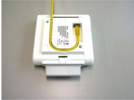
Figure 49: Cable at rear side of the cabinet
