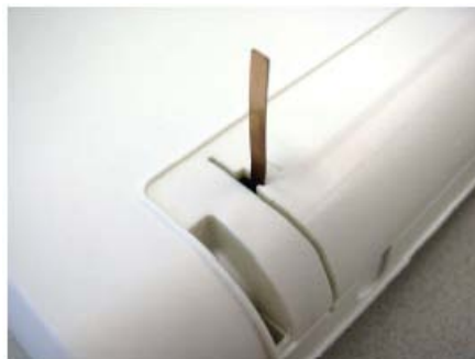
Figure 45: Antenna in locked position
