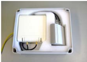
Figure 81: Antenna does not fit into the hole
