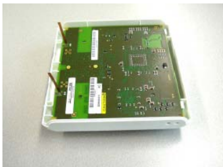
Figure 43: Bend Antennas carefully into vertical position
