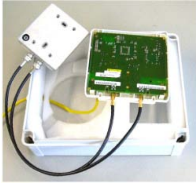
Figure 80: Connecting the cables to the 4720E
