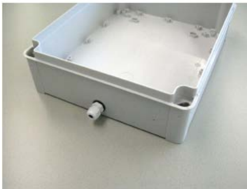
Figure 63: Swivel mounted to the cabinet
