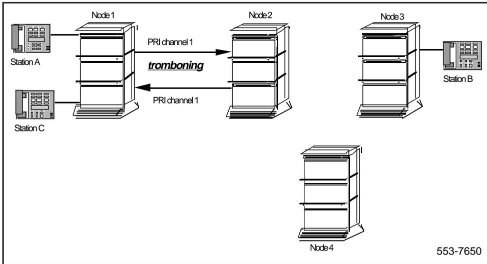
As soon as RO is completed, the RO/TAT initiates TAT at gateway Node 2. After TAT has been completed at Node 1, Node 2 simulates a transfer message to both Station A and Station C. This allows the Network Call Redirection feature to update the displays.
