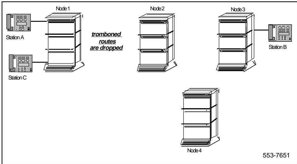
**Note:** If Station A is an attendant, and the Network Attendant Service feature is configured, Station B cannot transfer to Station C, and no optimization can take place. If NAS is not configured, Station B may transfer to Station C, and optimization will take place as described in this example.
