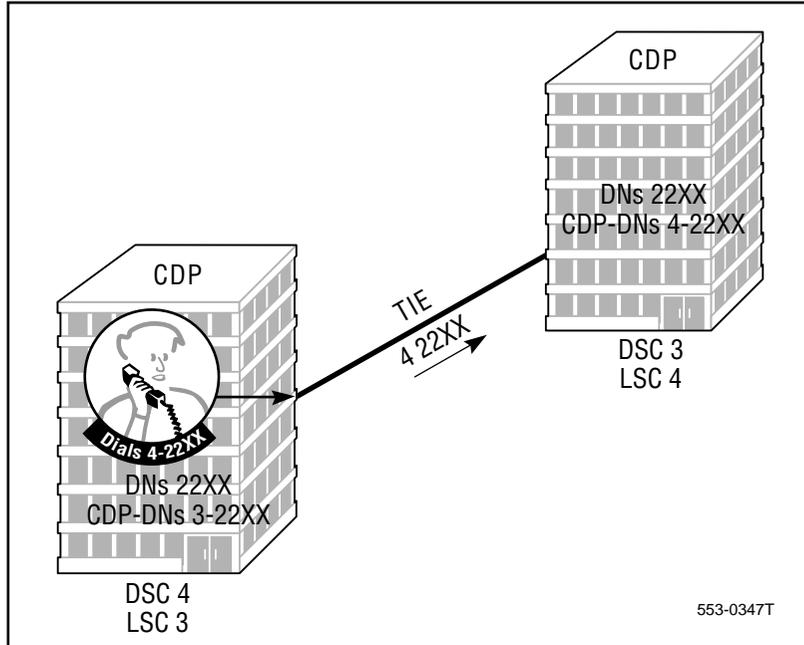
As you can see in the previous illustration, the DNs at the two switches are in the same number range. If neither switch administrator is prepared to change the DNs at their site, then the CDP dialing plan will have to be adjusted to make the CDP DNs unique at each site.
