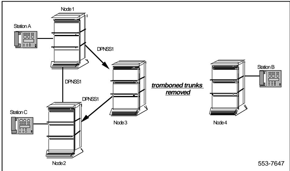
When TAT is completed on the MCDN side, The RO/TAT Interworking feature initiates RO on the DPNSS1 side by simulating a transfer at the gateway Node 3. The Three Party Service feature initiates signaling to update displays. Then, RO is initiated at Node 1, the originating node. The DPNSS1 trunks are dropped between Node 3 and 2 and Node 3 and Node 1, with Station A and Station C being connected over one DPNSS1 trunk.
