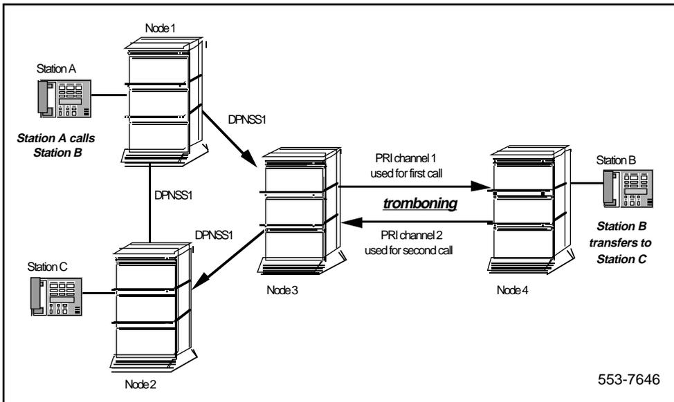
**Note:** The Network Call Transfer/Three Party Service gateway is not supported at the gateway Node 3. Therefore, RO is not initiated at Node 1, and the non-optimized DPNSS1 trunks remain connected.
