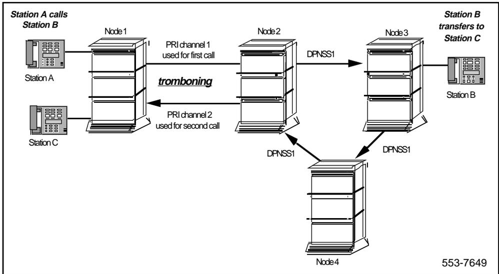
Once Three Party Service messaging has taken place, Node 2 initiates RO. The initial DPNSS1 routes are cleared. Node 2 becomes a MCDN/MCDN transit node, and the two tromboning PRI routes between Node 2 and Node 1.
