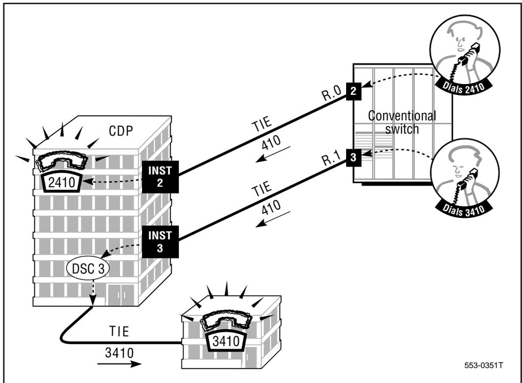
The cost of the TIE trunk routes required for this work around solution may be greater than the cost of implementing CDP software. Having several TIE trunk routes to the same destination is a very inefficient configuration. You will need fewer TIE trunks if they are collected together into one route as they would be if CDP software is installed.
