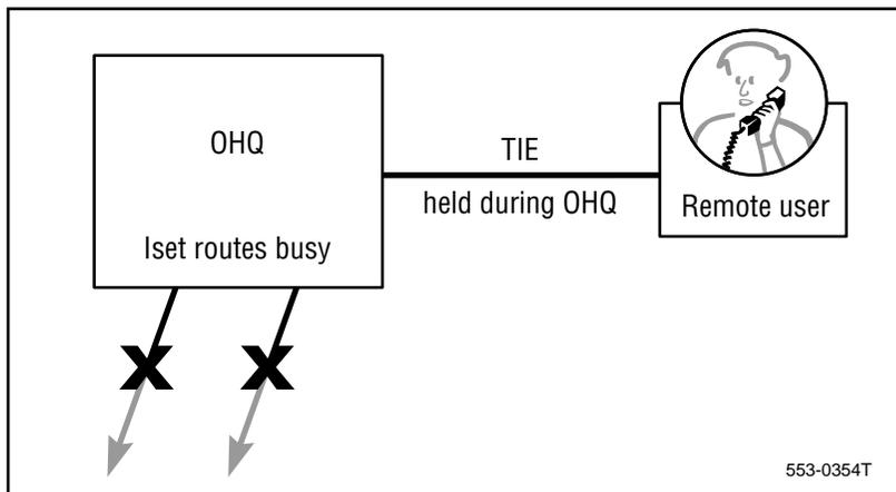
Also, as a call progresses through the network, OHQ can be offered to the call originator from any of the ESN nodes or ESN Mains that are used to process the call. As a result, OHQ can be offered more than once for a given call.
