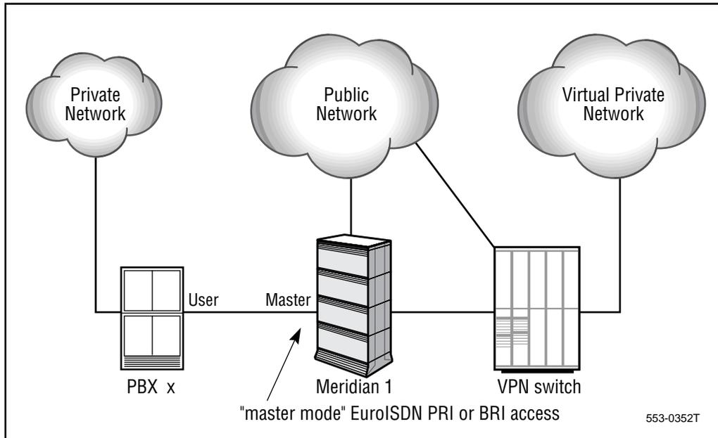
**Virtual Private Networks** offer network users reduced telephone bills by using their VPN network instead of the public network. The Meridian 1 may be used as a “remote point of presence” (RPOP) in a VPN, closest to the customer premises. It supports many different trunk connectivities and it has a lower cost than a public network switch.
