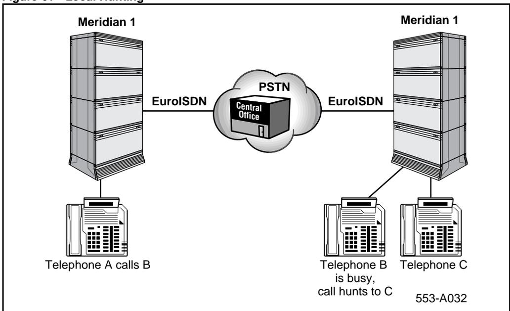
Figure 61 illustrates an incoming EuroISDN call with BNE Name information and a private CLID that redirects to telephone C when telephone B is busy. As soon as telephone C rings, the name and private number associated with telephone A display on telephone C, according to the presentation programming of telephone A. The name and private number associated with telephone C are delivered to telephone A.
