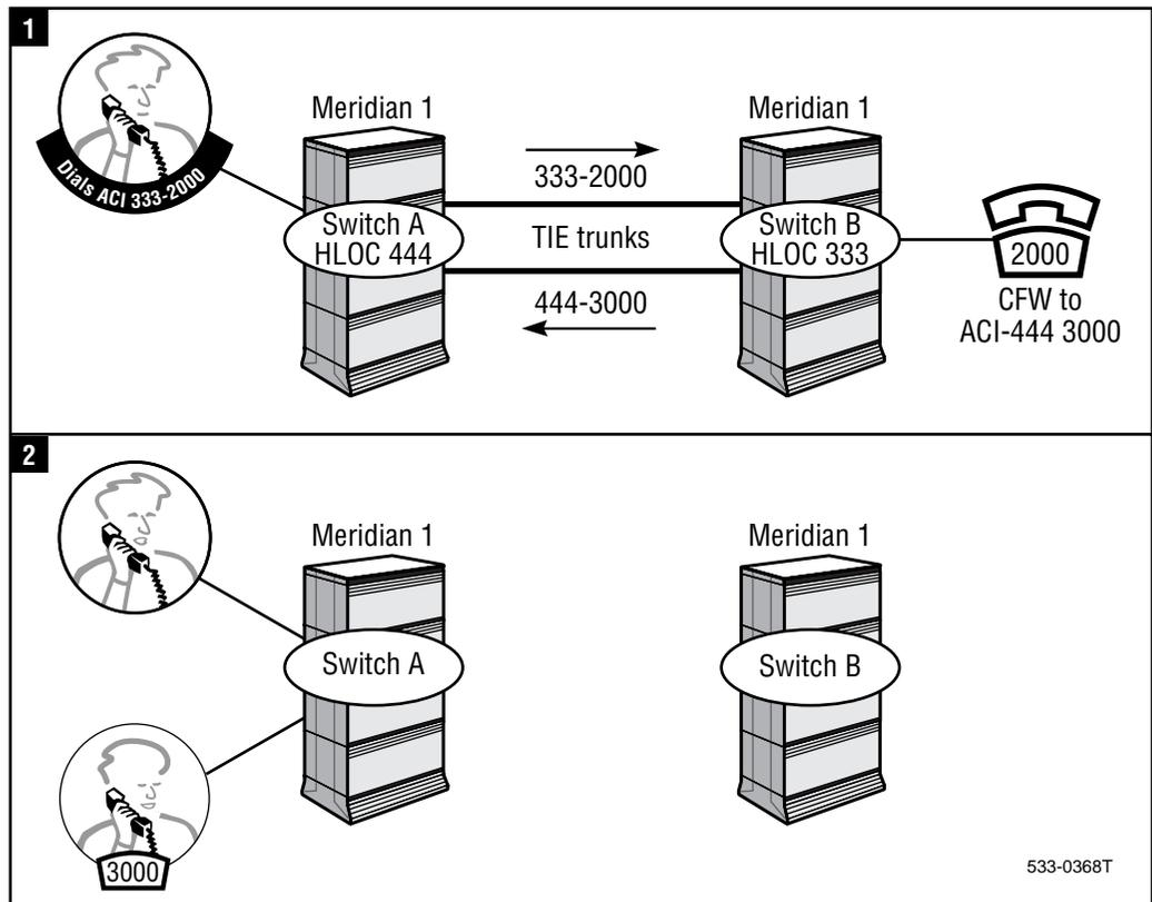
This capability is supported over ISDN PRI, ISL and VNS networks using MCDN protocols. TAT will be performed on VNS BRI trunks but not other configurations of BRI trunks.
