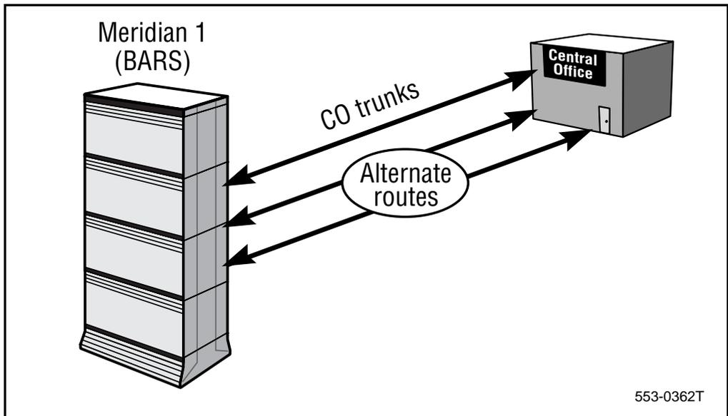
It is true that there are ESN networks where BARS has been installed at a switch performing as a node. This is not a supported configuration. This becomes especially important when the ESN network is being upgraded to ISDN functionality. The BARS software must be upgraded to NARS (or you can also choose BARS/NARS. Refer to the note marked \*\* under Table 30 that follows).
