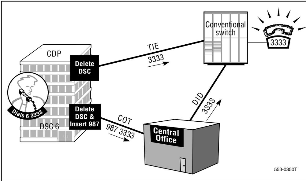
The users at the conventional switch will probably dial direct trunk access codes to make their calls. Train the users at the conventional switch to dial the TIE trunk access code followed by the CDP DN of the user they are trying to reach. If the conventional switch is connected to a node, then users should dial location codes instead of CDP DNs.
