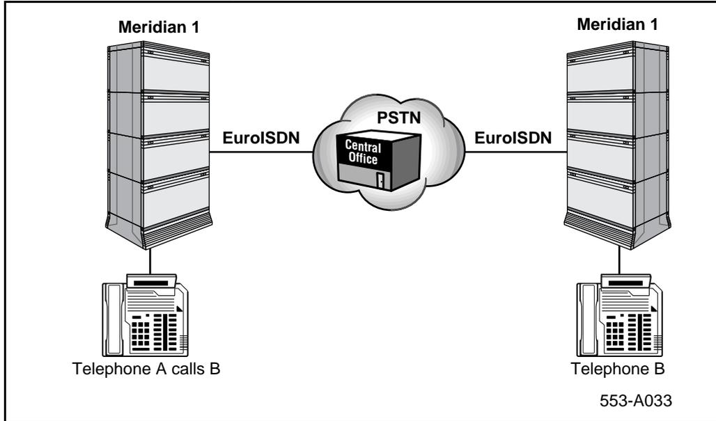
An outgoing EuroISDN call, carrying BNE signaling, as shown in Figure 62, is charged by the Central Office. If telephone A is a Meridian Modular Digital telephone and AOC Real Time Display is configured, the charge is displayed in the right corner of the first line, when it is received. The display of charge takes precedence over the display of name. The name displayed on telephone A is truncated if there is not enough space to display both the name and the charge.
