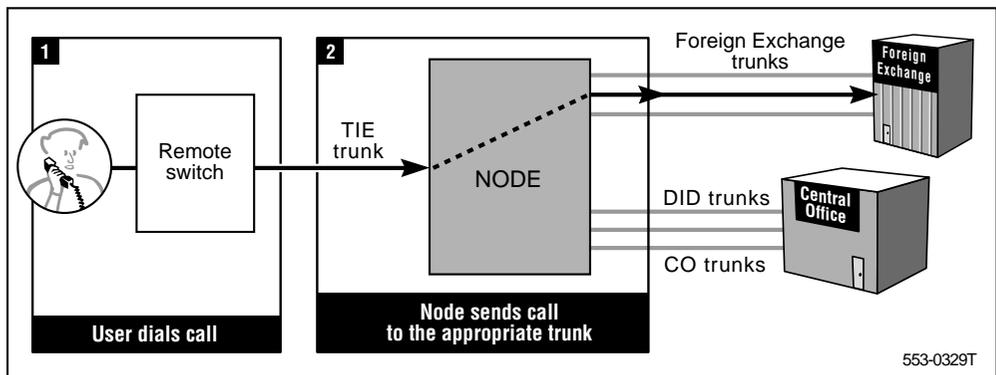
Networks are usually set up in such a way that there are clusters of remote switches connected to a central node.
