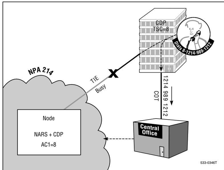
**Local Steering Codes (LSCs)** are designed to indicate the leading digit(s) of local DNs at a CDP switch. You may not need these if the local CDP DNs that a switch will receive are the same as the local DNs themselves.
