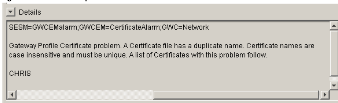
Figure 39 GWCEM Duplicate Certificate Alarm Detail
