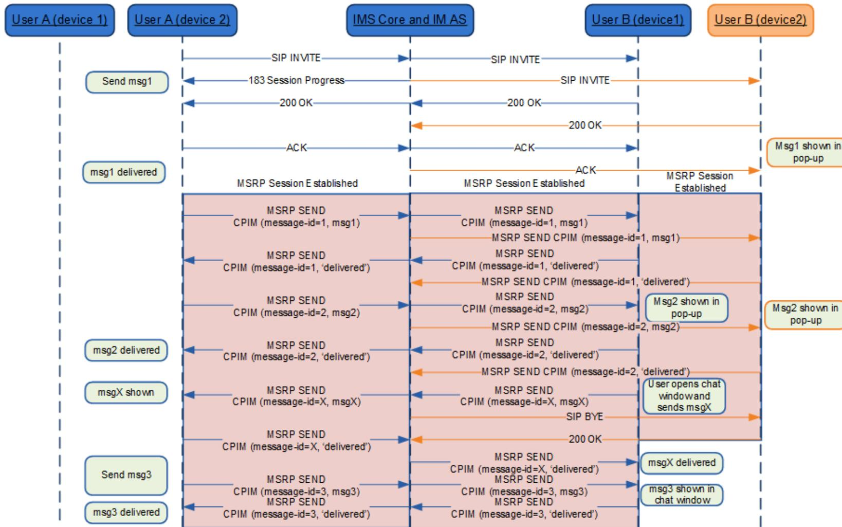
**Figure 38: Rejoin in active Chat which is torn down due to inactivity\***
