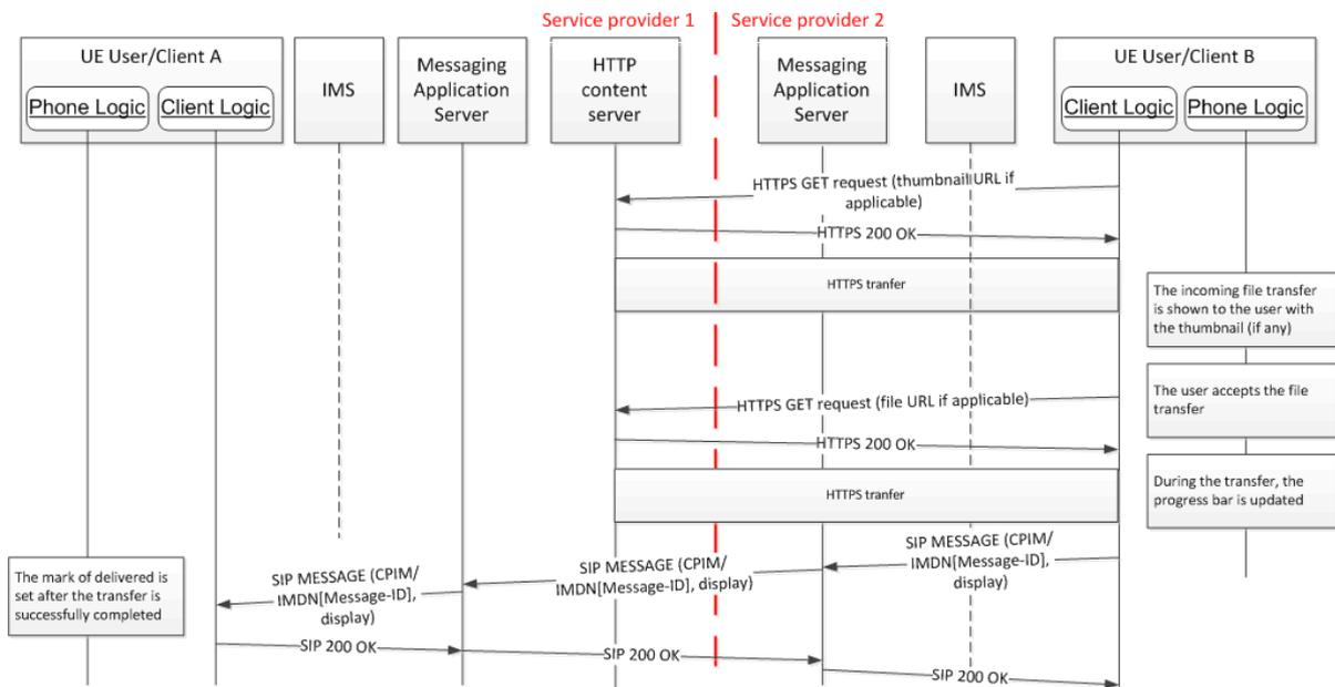
**Figure 11: File Transfer via HTTP: Receiver procedures**
