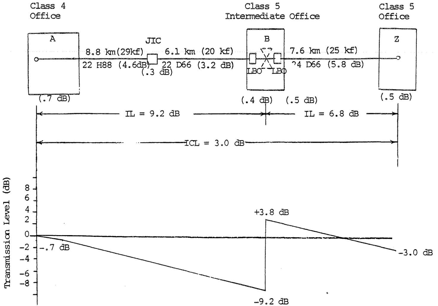
Figure 6. Toll Connecting Trunk and Level Diagram
