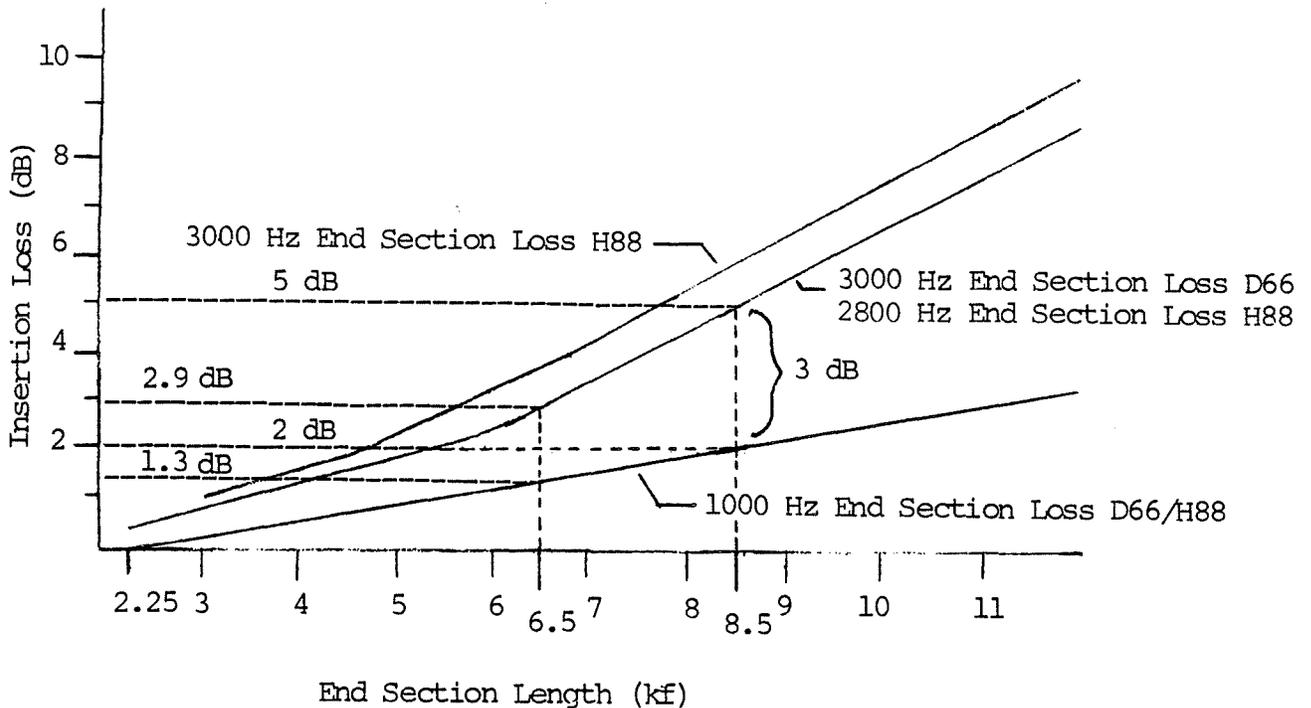
Figure 3. Average End Section Insertion Loss Between 900 Ohm Impedances for Different Lengths of D66 and H88 Loaded 24 Gauge Facilities
