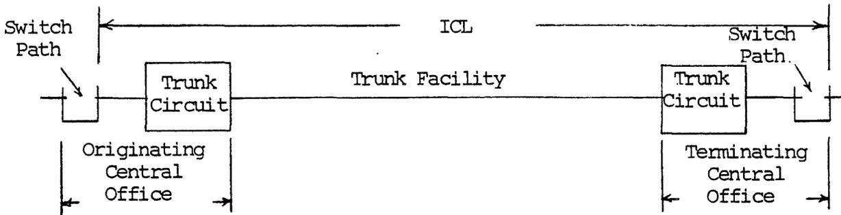
$$\text{ICL} = \text{Originating Office Losses} + \text{Trunk Facility Loss} + \text{Terminating Office Losses}$$
