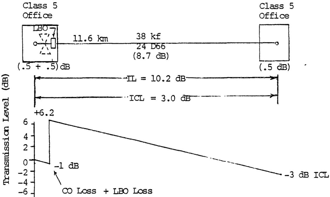
Figure 5. Local Trunk Circuit and Level Diagram
