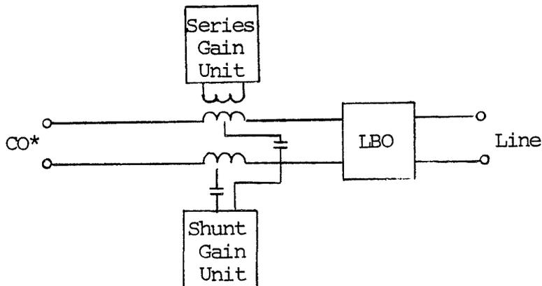
\* If used as an intermediate repeater (transmission line on both sides) an LBO is required at the CO side also.
