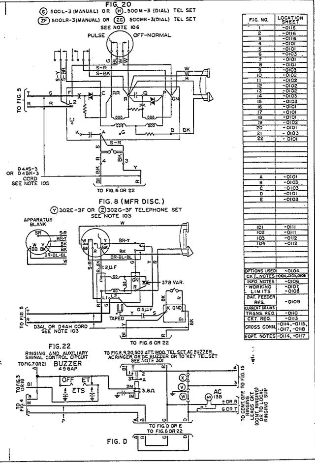
SD-65680-0101 PBX NO. 507A OR 507B STATION LINE, TRUNK, CONNECTING, TELEPHONE, RINGING, BUZZER AND 2WAY RINGDOWN TIE TRUNK CIRCUITS
