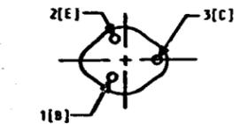
307. THE TERMINAL NUMBER ARRANGEMENT OF THE 51 AND 66 TYPE TRANSISTOR IS:
