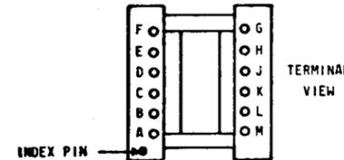
312. THE TERMINAL ARRANGEMENT OF THE 1300 TYPE INDUCTOR IS:
