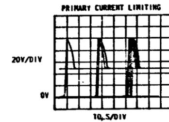
VOLTAGE ACROSS R601 TO  $V_{IN} (-)$ . THIS VOLTAGE IS EQUIVALENT TO THE COLLECTOR CURRENT OF Q401.
