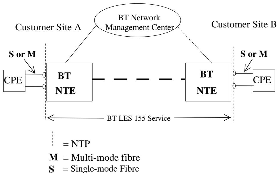
**Figure 1 - LES 155B Basic Element**
