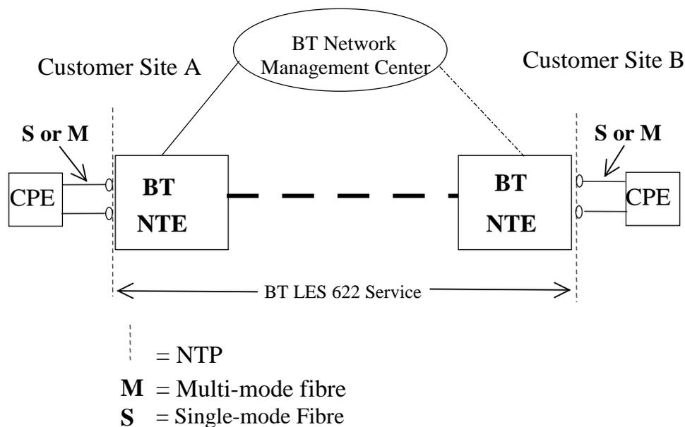
**Figure 1 - LES 622B Basic Element**
