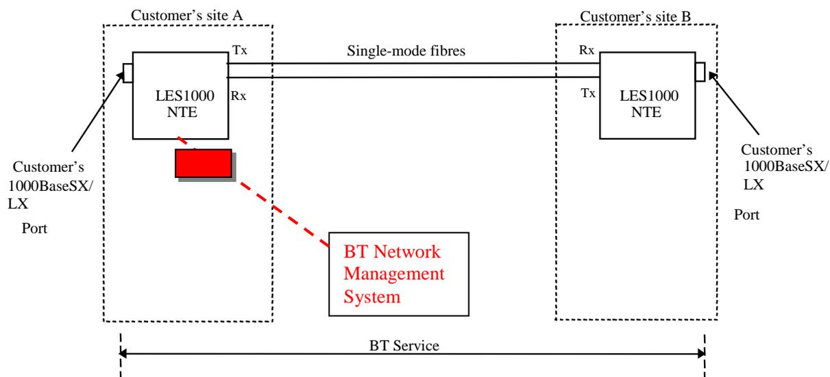
**Figure 1 Typical LES 1000 service configuration**
