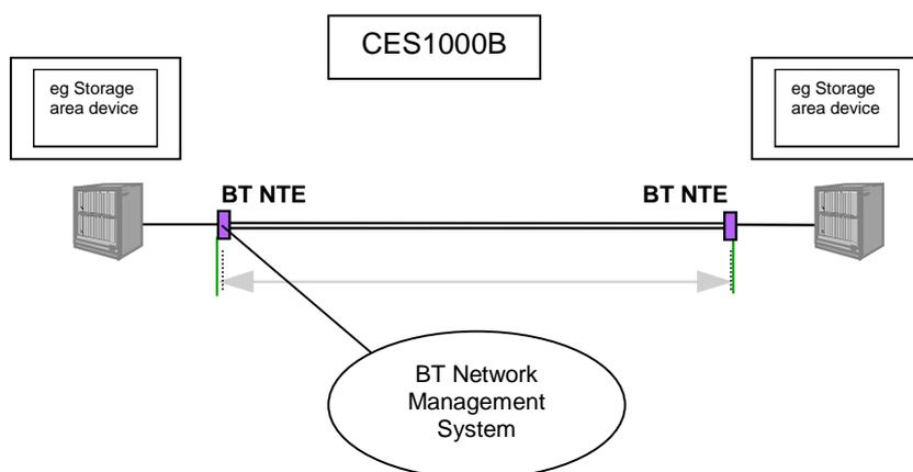
**Figure 1 Typical CES 1000 service configuration**
