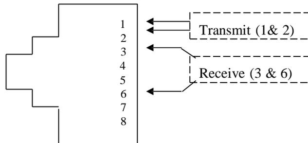
Figure 2. - WES 10/100 RJ45 Connector Pin Out Connections
