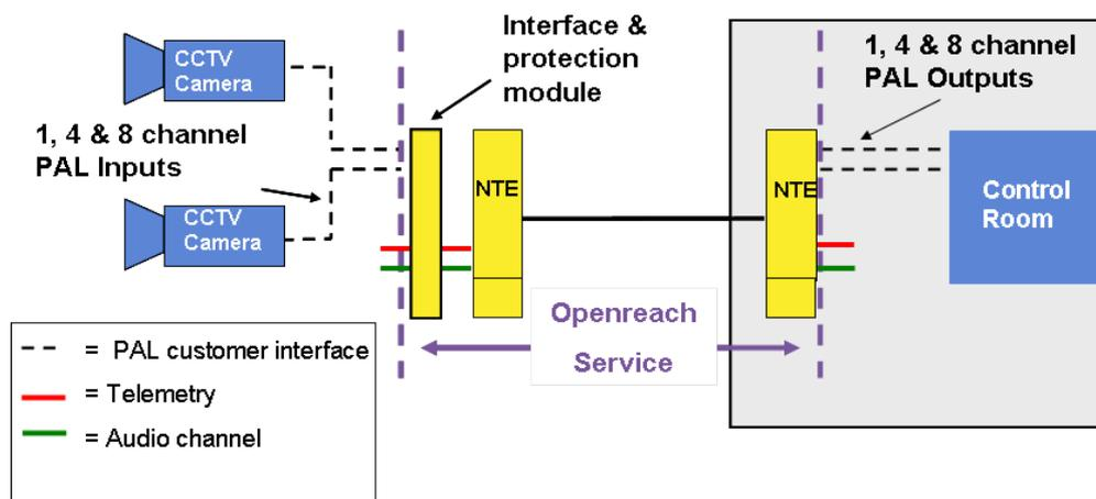
The CCTV Access uncompressed service has the option of a 1, 4 or 8 video channels. Audio and telemetry data channels are also provided.
