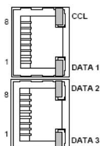
Note: Pin 1 of the RJ-45 socket is at the bottom of the connector.
