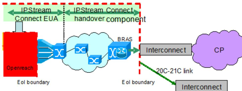
**Figure 1. Basic architecture of the BT IPstream Connect product**
