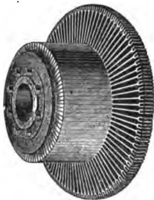
FIG. 18.—Commutator removed from armature shaft.
