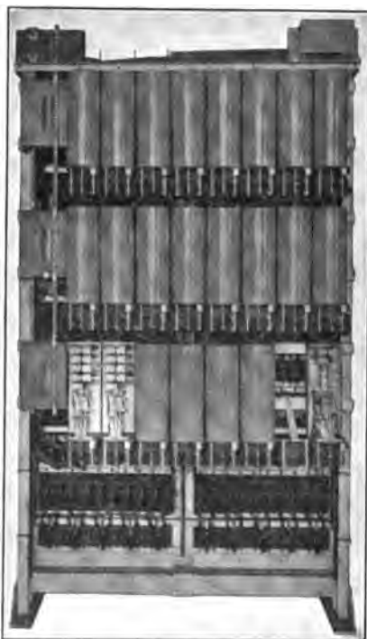
FIG. 90.—One-hundred-line switchboard, rotary lineswitches (back).
