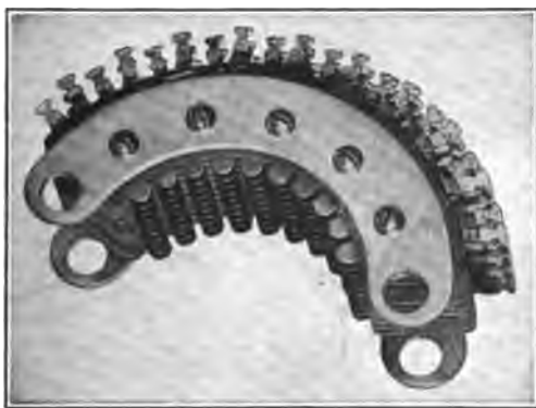
FIG. 55.—Connector-switch bank, unwired.
