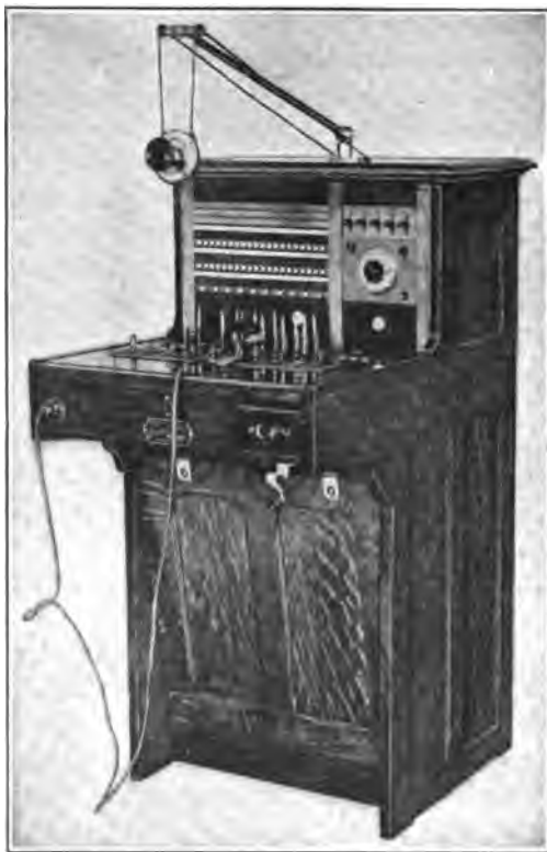
FIG. 157.—Private branch exchange switchboard.
