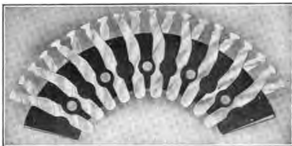
FIG. 56.—Detail of connector-switch bank.
