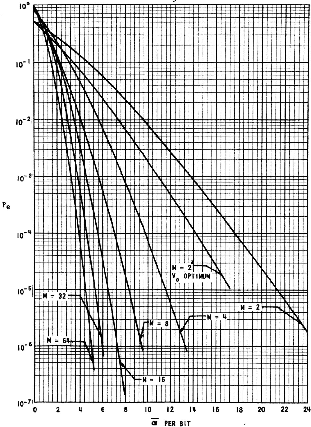
FIGURE 3 - PROBABILITY OF A SYMBOL ERROR  $P_e$  AS A FUNCTION OF THE AVERAGE NUMBER OF PHOTONS PER BIT ( $\pi = 4$ )
