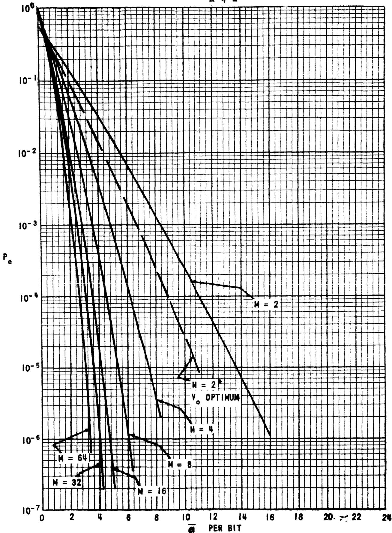
FIGURE 2 - PROBABILITY OF A SYMBOL ERROR  $P_e$  AS A FUNCTION OF THE AVERAGE NUMBER OF PHOTONS PER BIT  $\bar{n}$  ( $\bar{n} = \frac{1}{2}$ )
