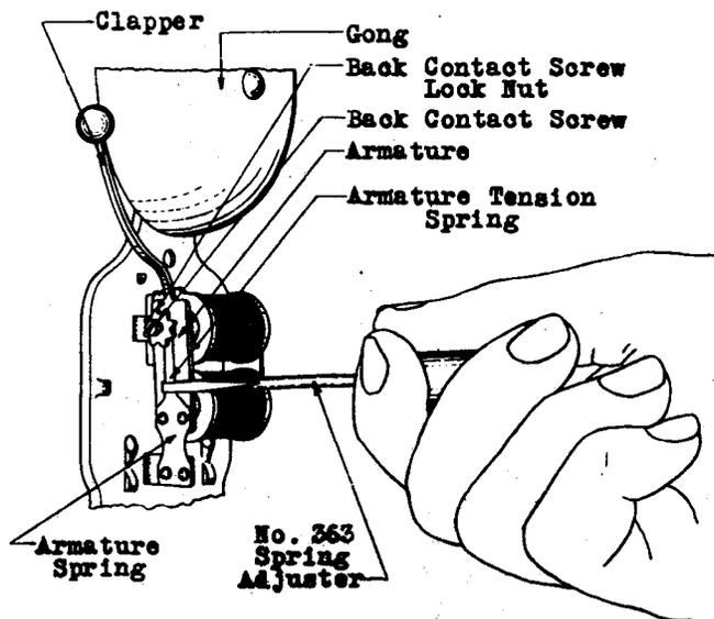
Method of Tensioning Armature Tension Spring
