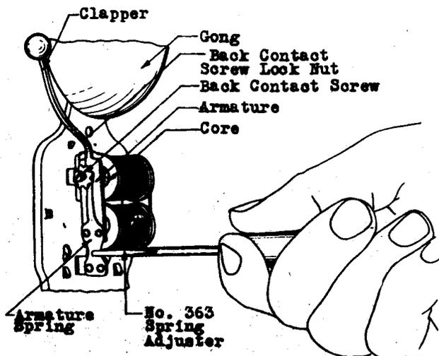
Method of Tensioning Armature Spring
