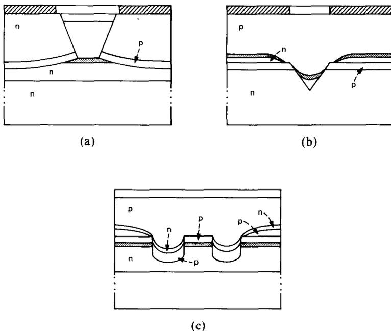
Fig. 9—The schematic cross sections of the (a) EMBH, (b) CSBH, and (c) DCPBH lasers are shown.
