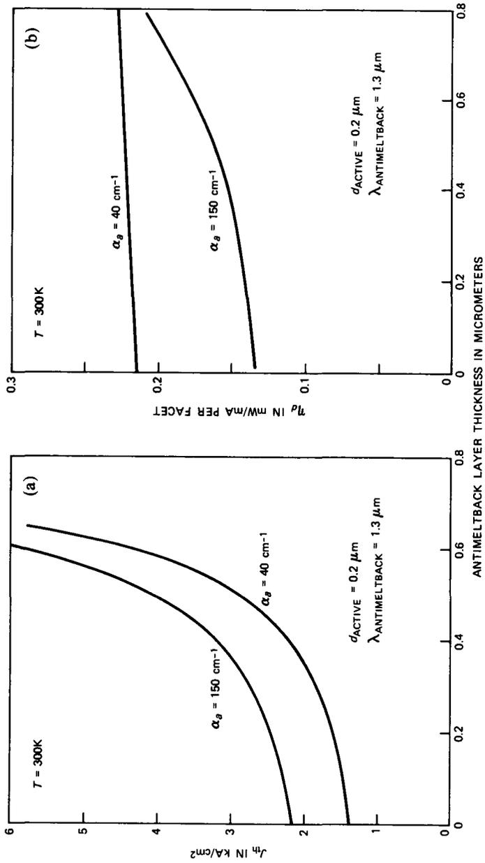
Fig. 8—The (a) threshold current and (b) external differential quantum efficiency as a function of the thickness of the antimeltback layer.
