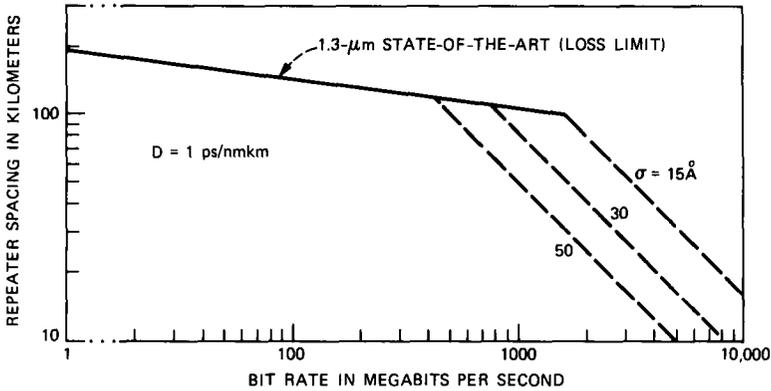
Fig. 15—Bit rate versus repeater spacing for lightwave systems operating near 1.3  $\mu\text{m}$ .
