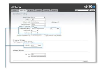
The Output Power, Antenna Gain, Cable Loss, and Frequency fields are provided to the professional installer to assist in meeting regulatory requirements.
