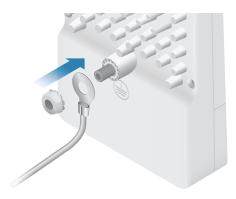
3. At the installation site, secure the other end of the ground wire to a grounded mast, pole, tower, or grounding bar.
