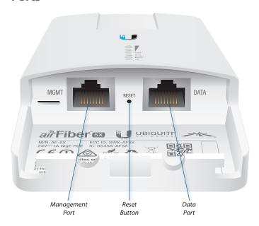
**Management Port** 10/100 Mbps, secured Ethernet port for configuration. *In-Band Management* is enabled by default in the airFiber Configuration Interface. When *In-Band Management* is disabled, the *MGMT* port is the only port that can monitor, configure, and/or update firmware.
