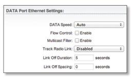
**DATA Speed** This is the speed of the *Data* port. By default, the option is **Auto.** The AF-5X automatically negotiates transmission parameters, such as speed and duplex, with its counterpart. In this process, the networked devices first share their capabilities and then choose the fastest transmission mode they both support.
