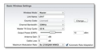
**Wireless Mode** By default, the Wireless Mode is *Slave*. You must configure one AF-5X as **Master** because each PtP link must have one *Master*.
