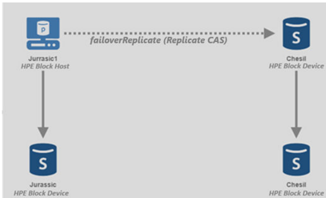
Figure 7: Dataflow with support for non-destructive test-failover (using refreshed replications)
