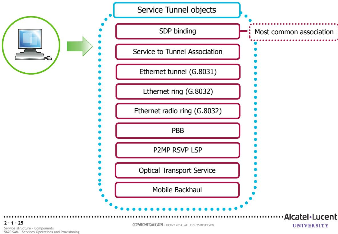
The most common type of tunnel used in 5620 SAM is a Service Distribution Point binding. Service tunnels originate on an SDP on a source NE and terminate at a destination NE. The destination NE directs packets from the service tunnel to the correct service egress interfaces (SAPs) on that device. Services that originate and terminate on the same NE do not require service tunnels, because the same NE is both the source and the destination.
