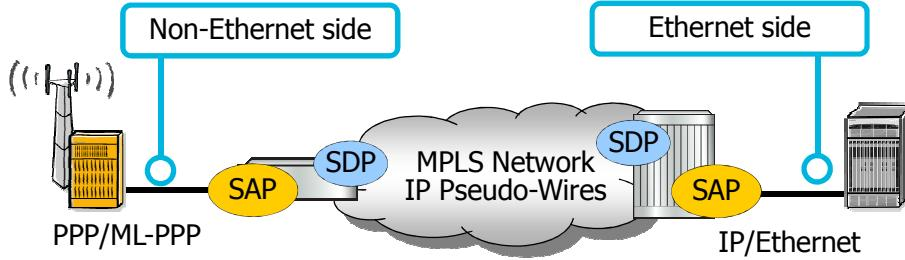
An Ipipe can provides IP connectivity between a host attached to a point-to-point access circuit (PPP) with routed IPv4 encapsulation and a host attached to an Ethernet interface.
