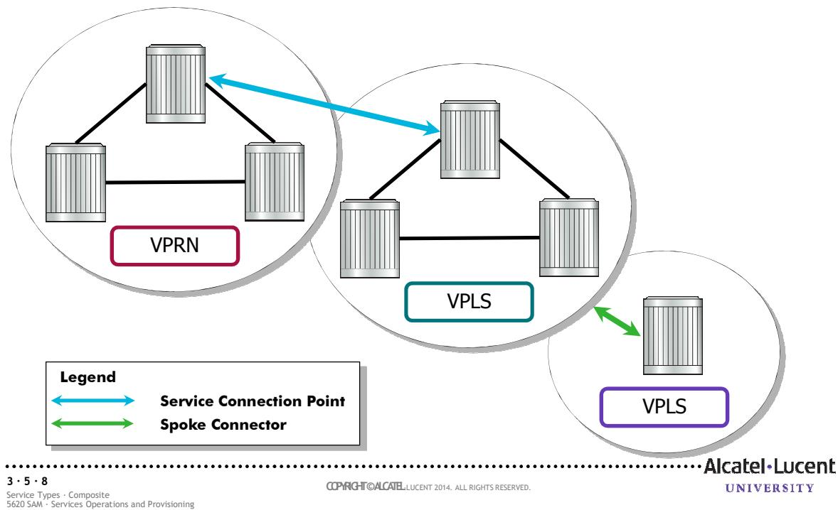
A composite service is a set of linked services whose function supports complex applications that require a combination of services, such as VLAN connections to an HVPLS, an IES spoke into a VPLS, or a VPRN-to-VPLS interconnection.
