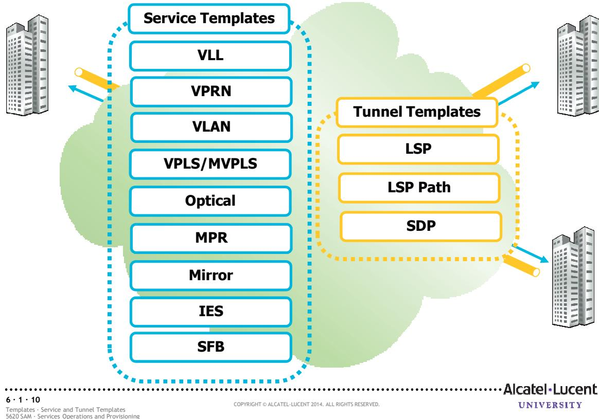
Service template configuration supports the configuration of multiple service types using XML API script-based templates.
