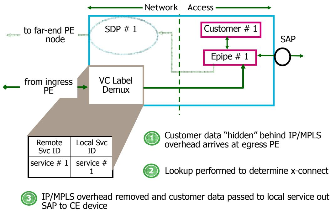
To be able to remove customer traffic from within the IP/MPLS and send it along to the CE device connected to the egress PE:
