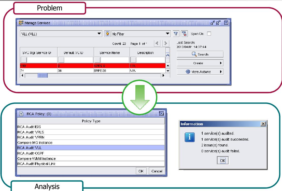
The 5620 SAM RCA audit tool allows you to perform on-demand or scheduled verifications of the configuration of services and physical links to identify possible configuration problems.
