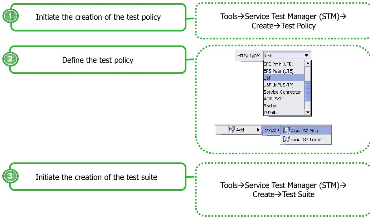
The workflow illustrated above describes the steps for a network administrator or operator to configure a generated STM test.
