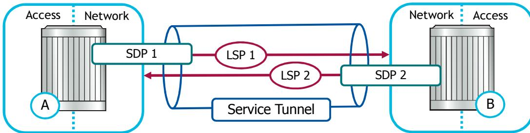
The operational theory of a service tunnel is that the encapsulation of the data between the two managed edge NEs appears as a Layer 2 path to the service data although it is really traversing an IP or IP/MPLS core.
