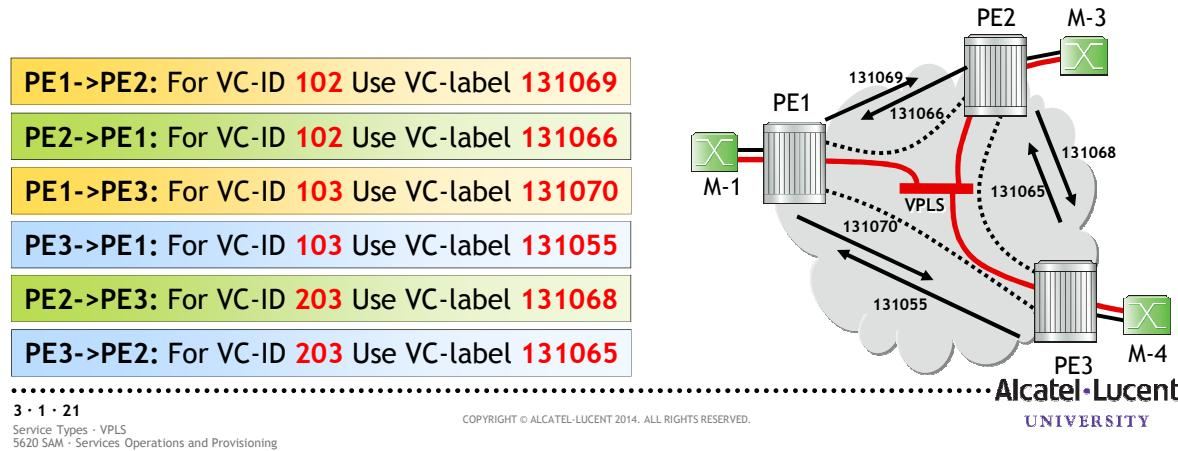
Customer packets are transported either inside an IP packet (GRE) or inside an MPLS packet.
