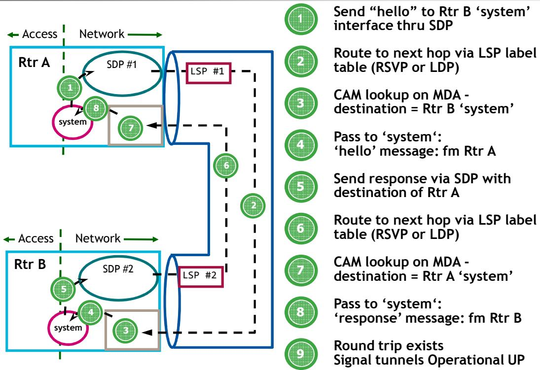
The diagram above illustrates the process for service tunnel signaling. In summary, the source router sends a connect message to the destination router system interface through the associated SDP. At the destination, the request is passed to the system interface which sends a response back to the source router through an SDP.
