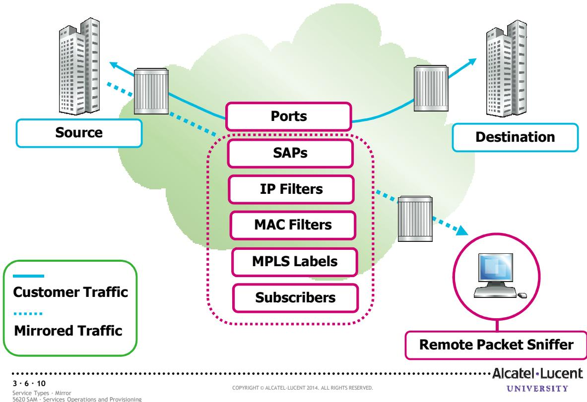
There are Layer 3 switches and routers from other vendors that provide service mirroring on a per-port basis within the device. The additional functionality provided by Alcatel-Lucent service routers is the ability to mirror on an n-to-1 unidirectional service basis and re-encapsulate the mirrored data for transport through the core network to another location using IP or MPLS tunnels.
