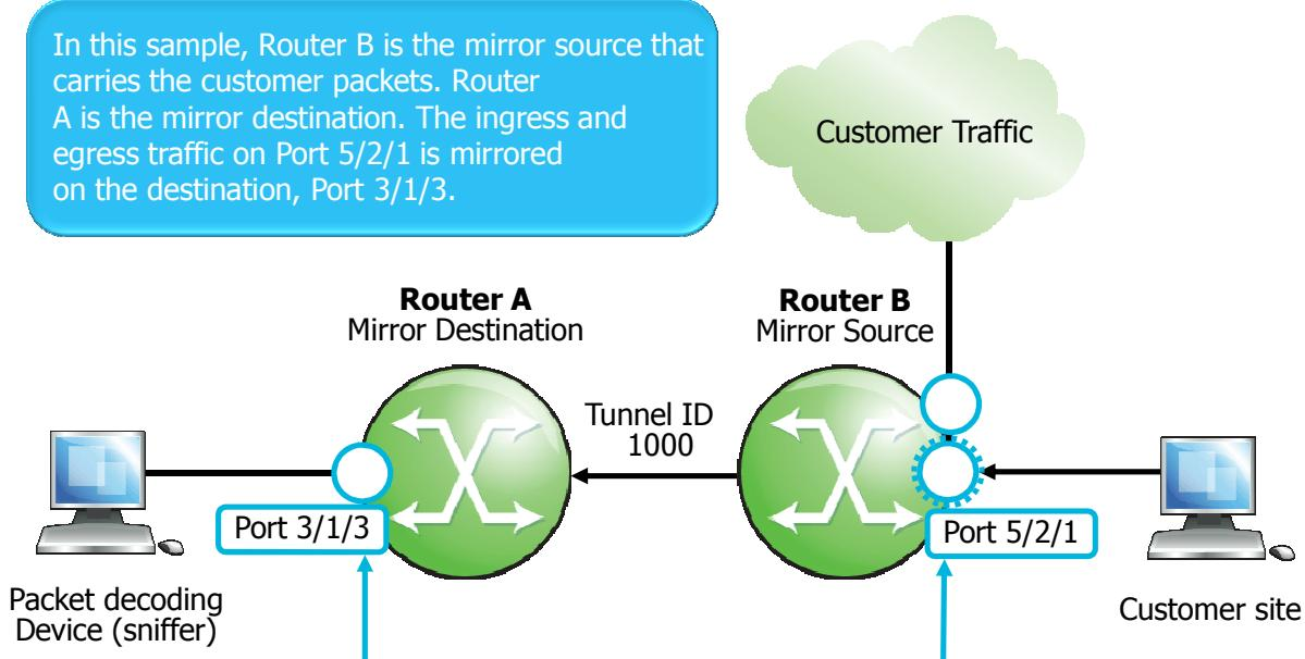
Configure a mirror service that specifies the source and destination parameters
