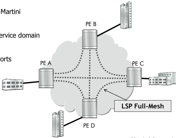
For each VPN at each site, a Customer Edge (CE) device connects to the Provider Edge (PE) router via a point-to-point access connection.
