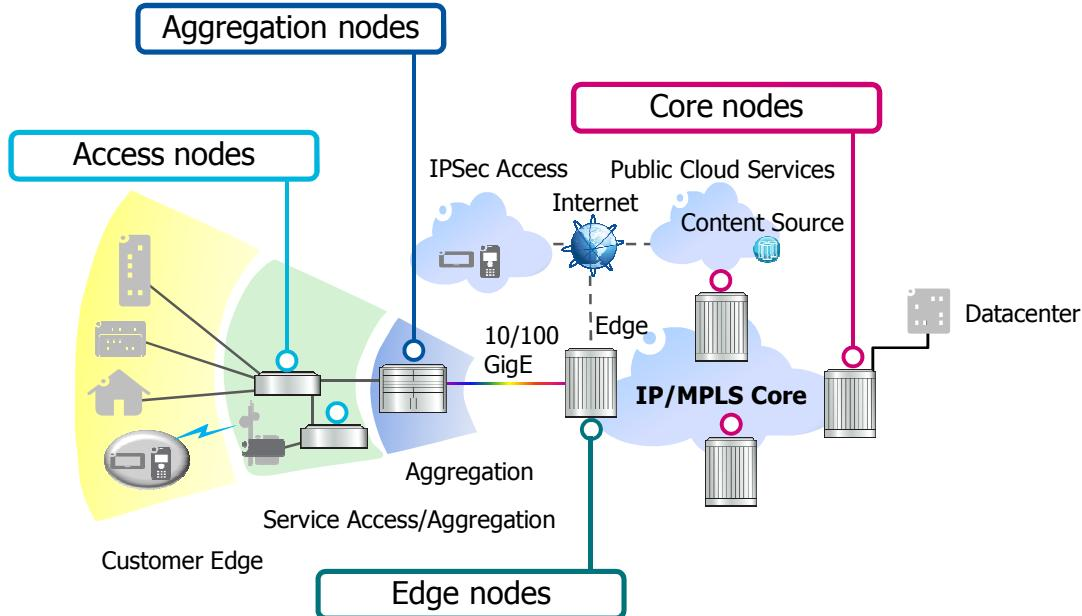
**Access nodes**, in general, do not need very high capacity or very high processing power since they will be dealing with a reduced number of traffic streams, and therefore a reduced number of configured services (as compared to nodes at the network's edge). What they do need, however, is to be compatible with whatever technology the customer has implemented.
