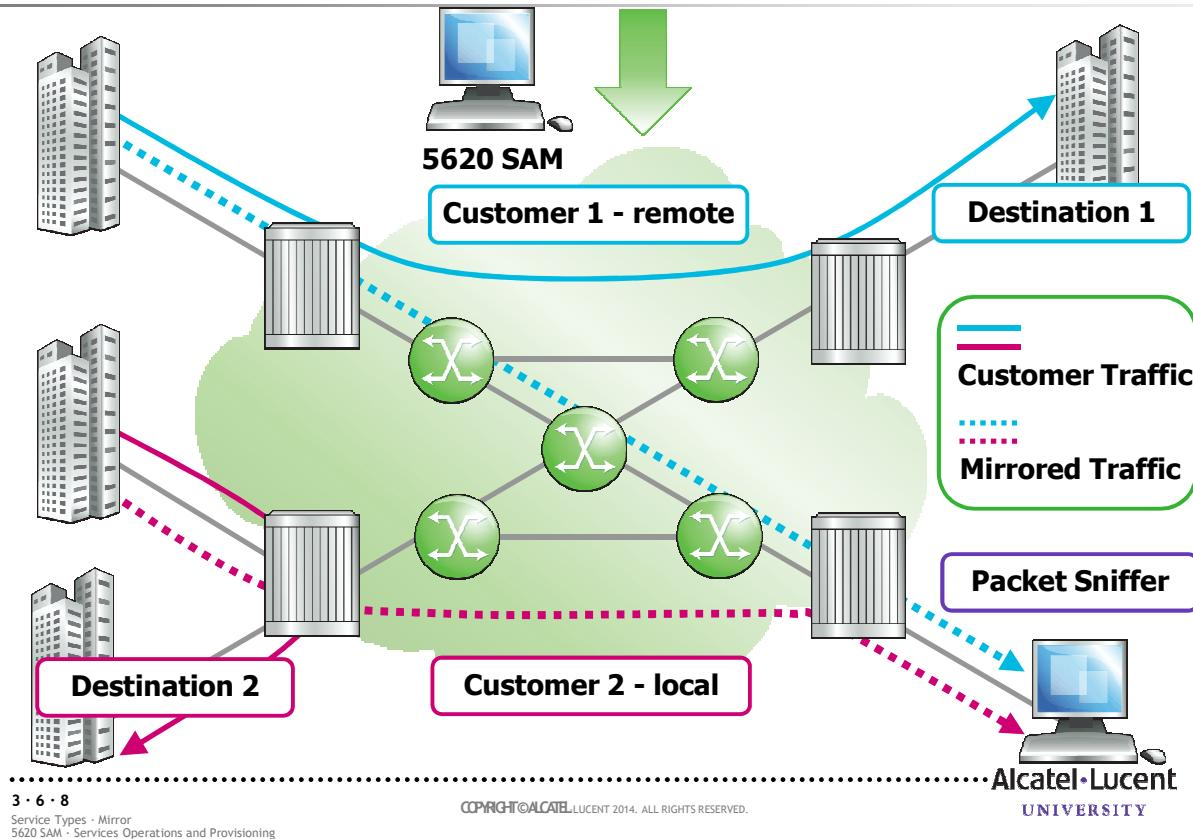
The 5620 SAM GUI implementation of service mirroring provides mirroring of service traffic packets from any service type.
