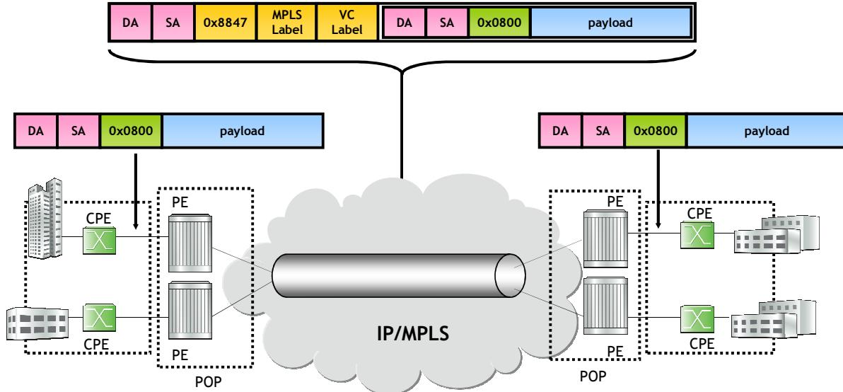
**The customer frame becomes the payload of the MPLS frame**
