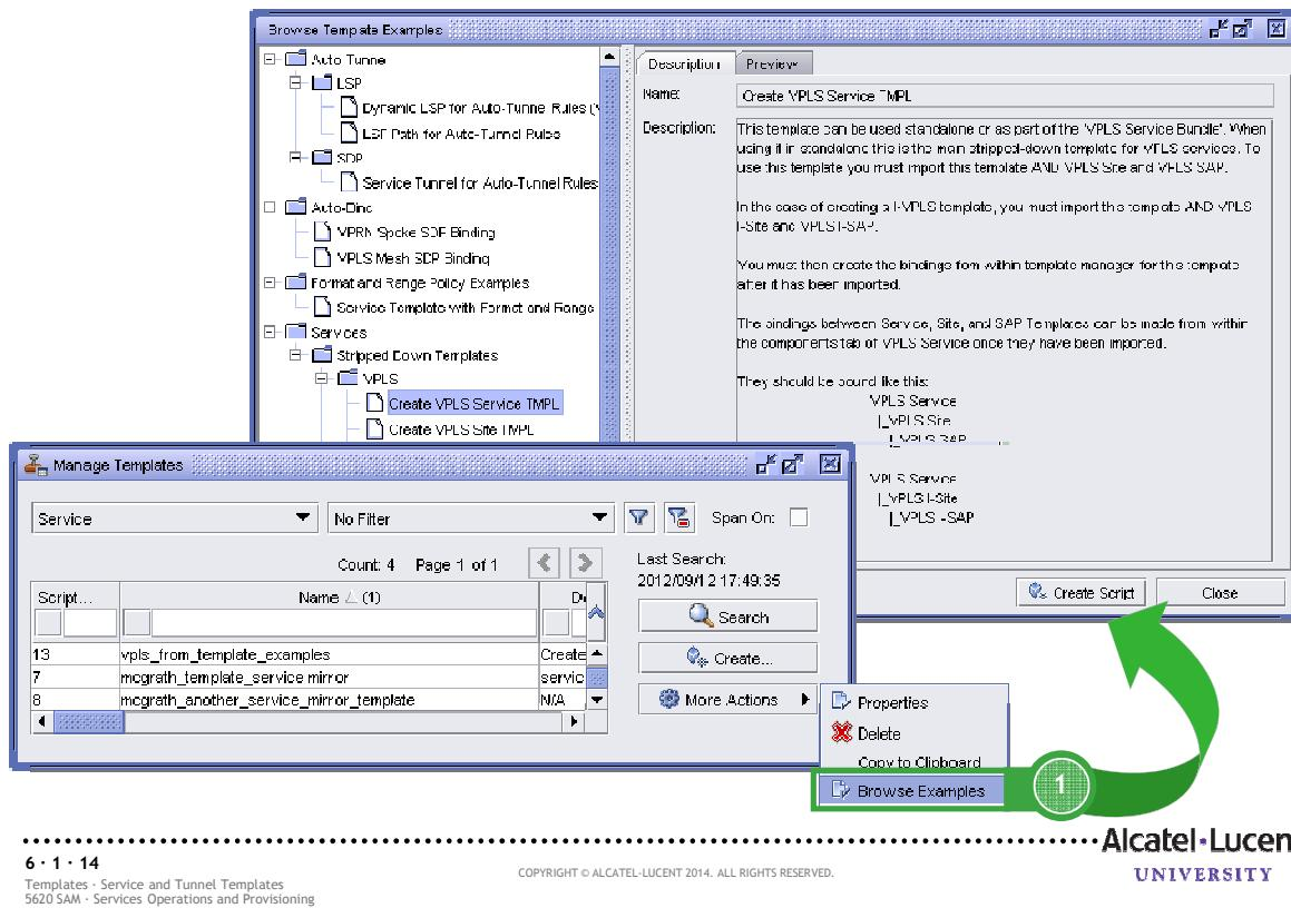
Service template examples provide a way for users to learn the procedures, practices and concepts that are required to configure XML API templates; for example, creating a VPLS service template. The preview tab allows you to view the example script.
