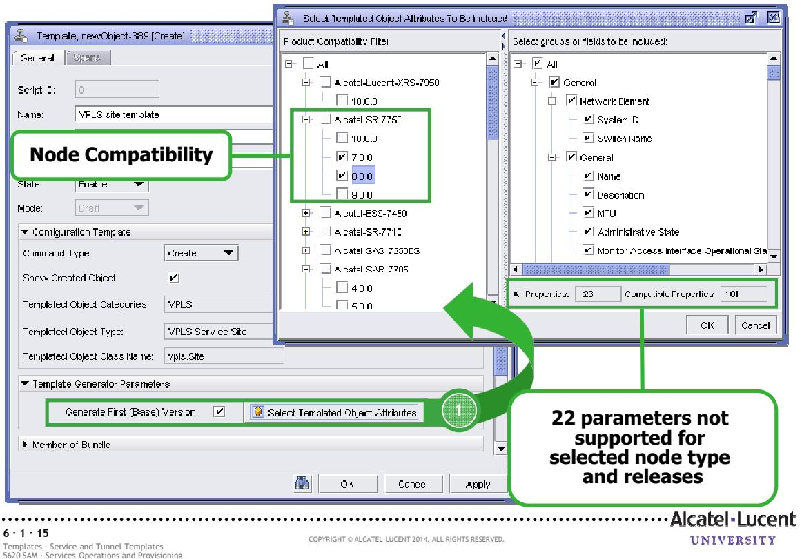
The Parameter Selection Form allows users to specify the node release types and versions that are specific to the template. The generated template supports the configuration of parameters that are supported on all node release types and versions that are associated with the template. Any parameters excluded from the template but supported on the node can be configured using the object properties form.
