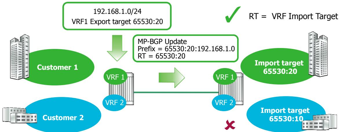
Routes are tagged with a route target value before sharing them with remote PEs due to the VPRN configuration (vrf-target parameter). Alternatively, export policies can be defined to add route target values (community attribute) to a route advertised to remote PEs. Upon receipt of a VPN-IPv4 route, a PE router will by default add the route to the VRF associated to the route target value received with the route. Import policies can be used to decide whether to add a given route to a VRF.
