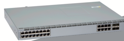
720XP-24ZY4 16 100M-2.5G PoE Copper Ports 8 100M-5G PoE Copper Ports 4 25G 25G SFP
