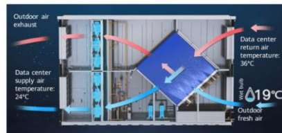
Hybrid mode (fan, water pump, and compressor started)
