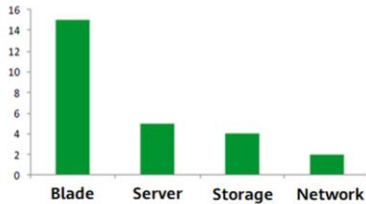
Typical power density of different types of cabinets
