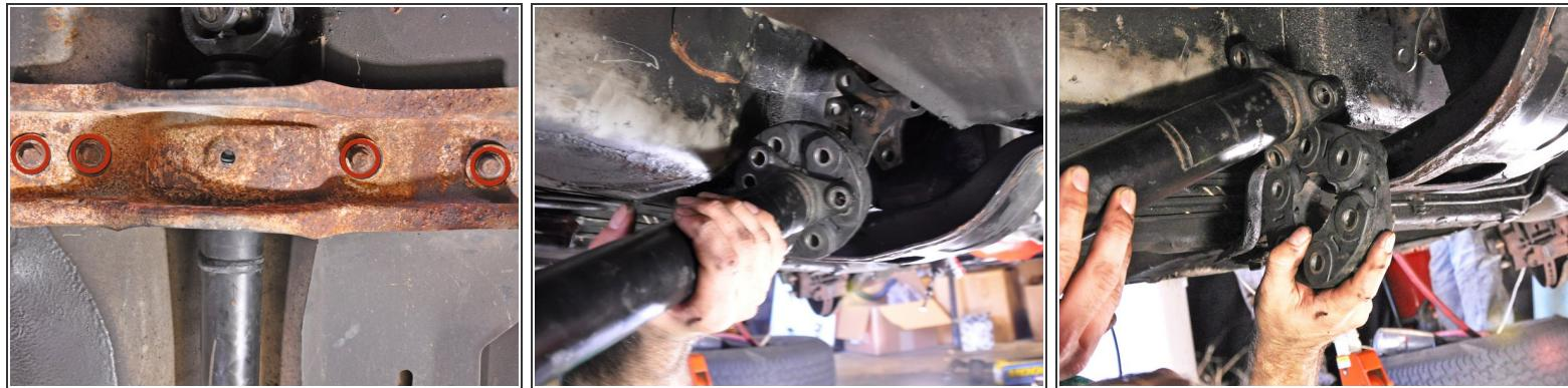
**⚠** Support the drive shaft with a jack, jack stand, or other prop so it does not fall and get damaged or injure someone when the support is removed.
