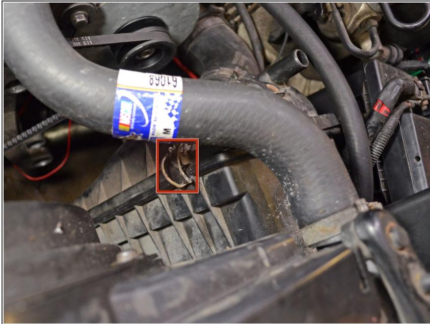
*i* The engine air filter housing is located at the front of the engine bay, between the engine and the radiator.
