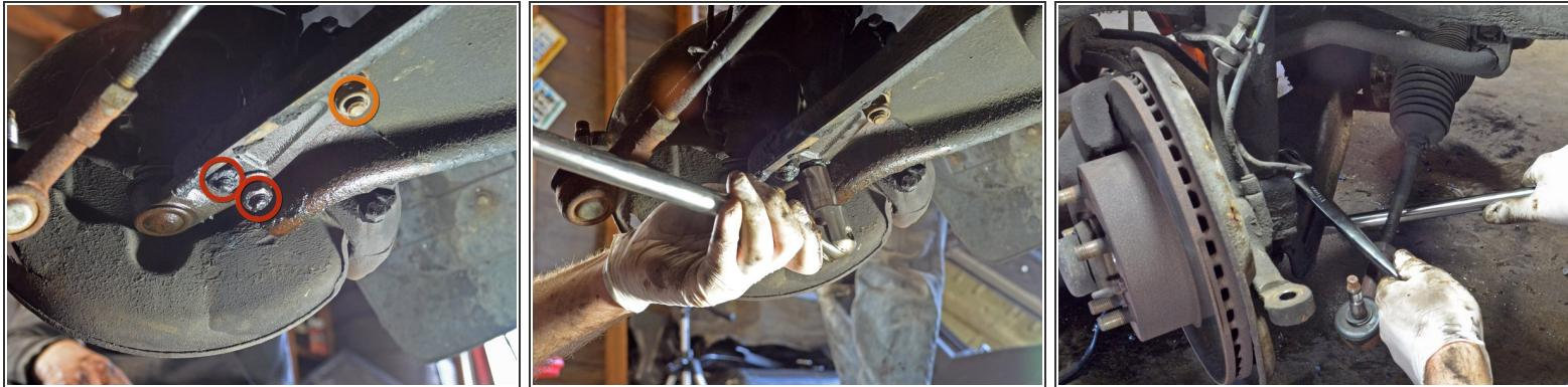
**i** The ball joint is held to the control arm by three 18 mm bolts.
