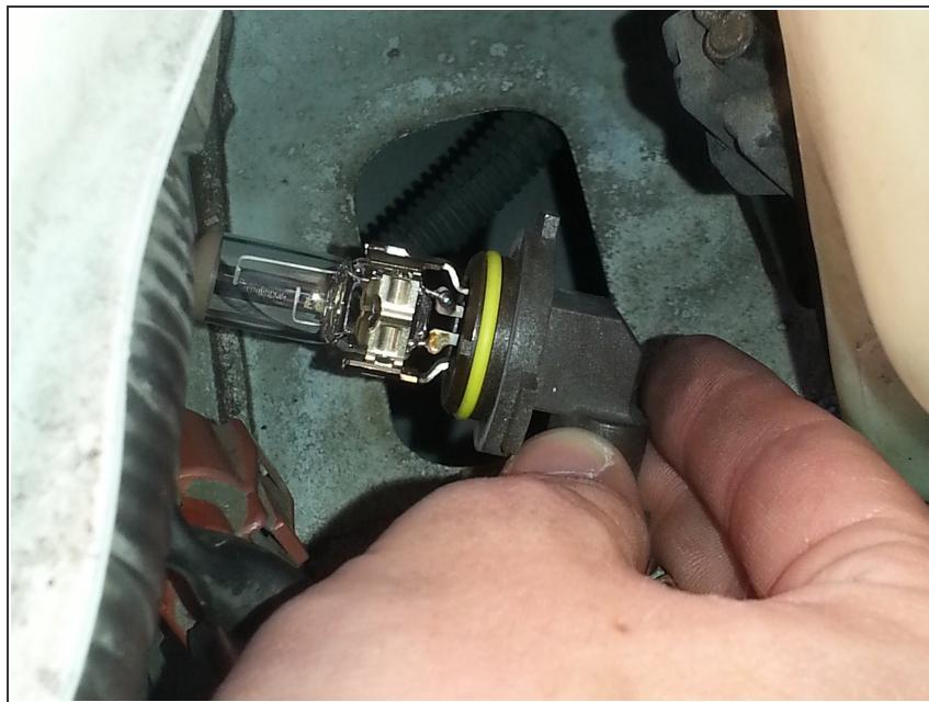
ⓘ With bulb exposed, twist broken bulb counterclockwise to unscrew from electrical connection. Screw in new bulb clockwise and replace back into socket.
