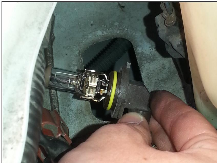
⚠ Be very careful twisting new bulb into electrical connection as the bulbs are very easily damaged.
