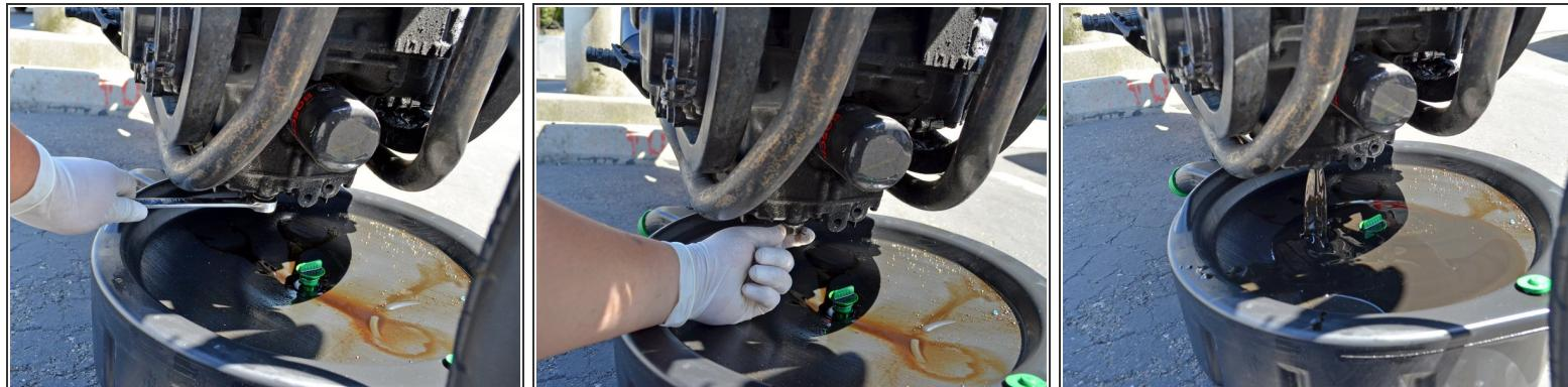
**⚠** Always wear protective gloves and eyewear when working with motor oil. Be careful if your bike has been running recently as the engine and exhaust may be very hot. Keep rags or towels nearby to wipe up any spills.
