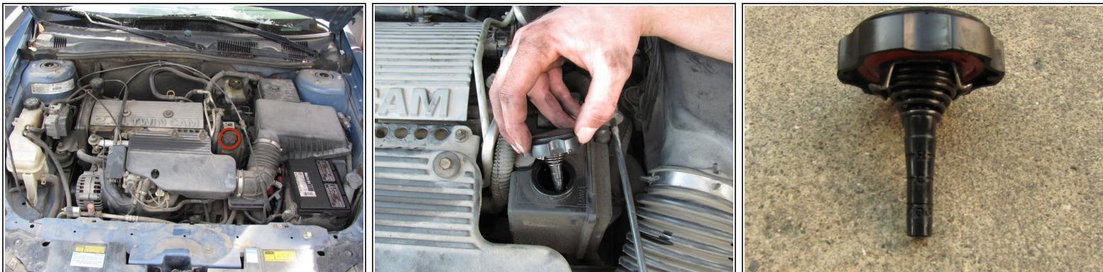
**⚠** Do not overfill the power steering fluid reservoir, as this can overwork the power steering pump and cause it to burn up.
