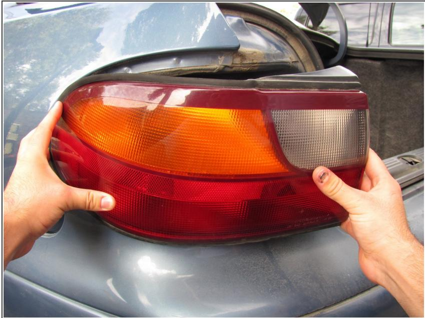
⚠ When the tail light assembly comes loose, do not fully remove it because it may damage the connected wires.
