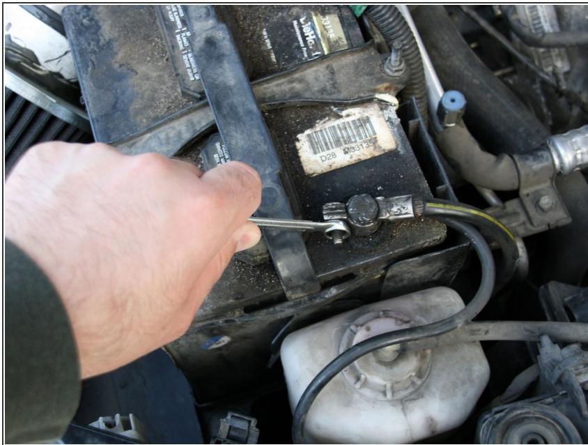
⚠ Before going any further: disconnect the battery. I keep a 10 mm wrench in my center console specifically for this purpose.
