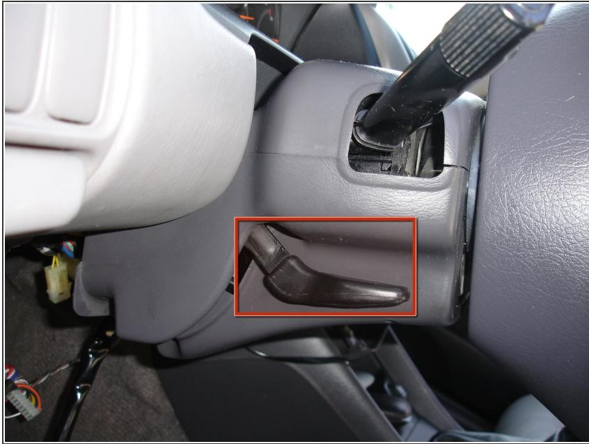
ⓘ Of course proceed at this point only if the switch failed one of the continuity tests. Also, make sure that the ignition switch is in the "Lock" position before proceeding any further.
