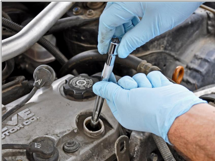
**(i)** It is easiest to accomplish this step with the socket wrench disconnected from the extension.
