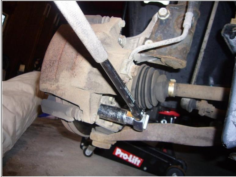
**⚠** After jacking up the car PLACE JACK STAND(S) under the car for safety, THEN take off the wheel.
