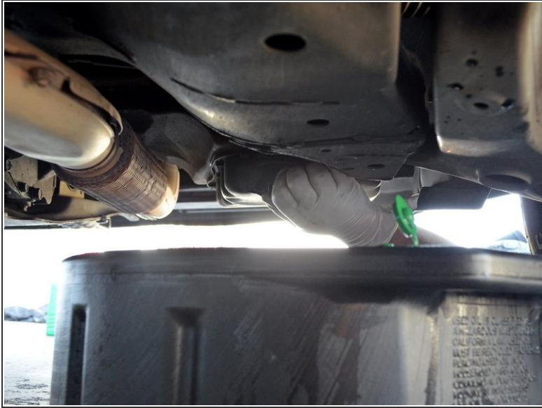
**⚠** Always wear protective gloves and eyewear when working with motor oil. Be careful if your car has been running recently as the engine, transmission and exhaust may be very hot. Keep rags or towels nearby to wipe up any spills.
