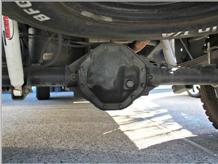
**⚠** When tightening the bolts on the diff plate it is vital that you tighten them in a star pattern to avoid warping the plate. Do not exceed a torque of 40 ft-lbs per bolt.
