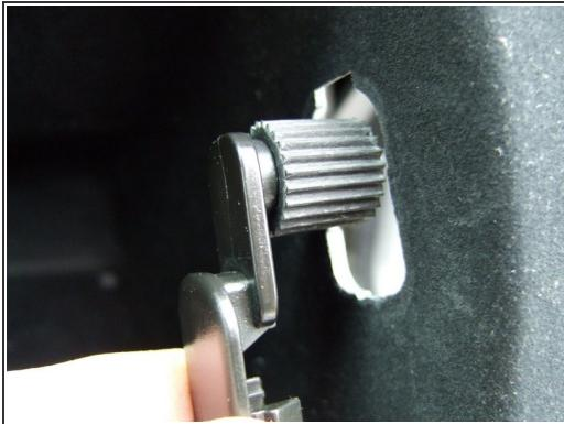
ⓘ On the Honda Accord and other models, the glove box incorporates stops in the box drawer itself. Not the TSX! The glove box has two stops, left and right side, that must be removed.
