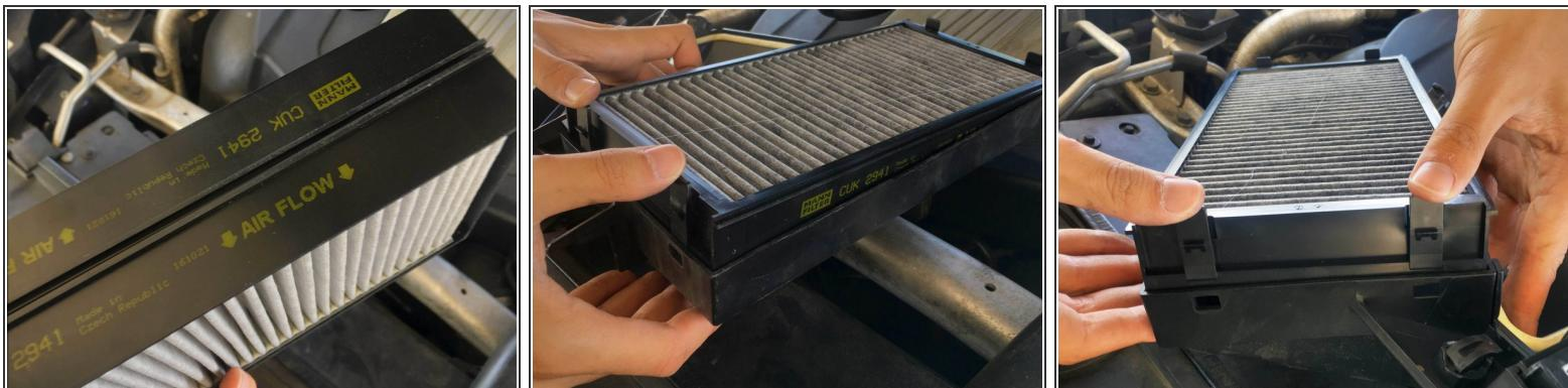
★ Pay attention to Air Flow indicator arrows when reinstalling the filters.
