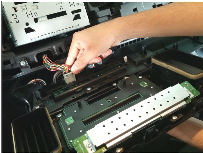
*(i)* Optional: If you choose, you can remove the harness shown. (See directions on Step 12 for removing a harness clip.) Otherwise you can simply rest the fixture on top of the shift knob.
