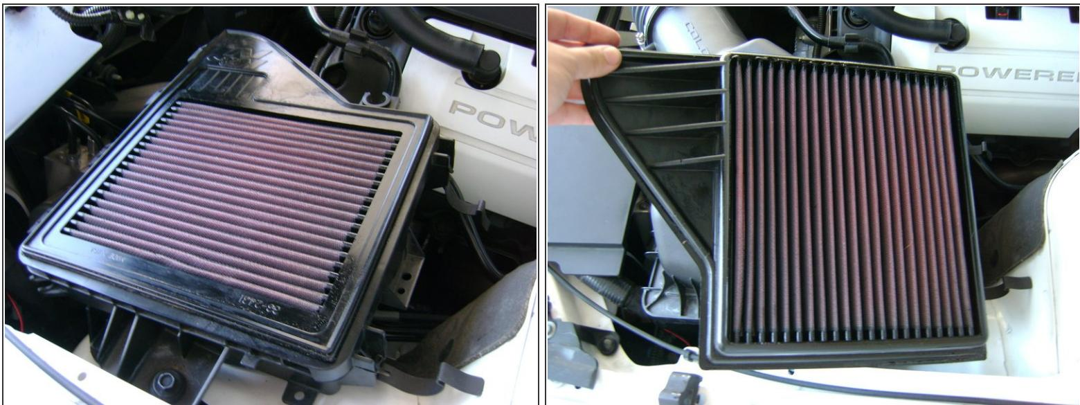
*(i)* Make note of the orientation of the air filter before removing it.
