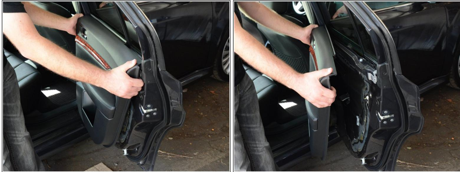
*(i)* The door panel should now be loose on all sides — but do not pull it off completely just yet! There are cables attached to it on the inside.
