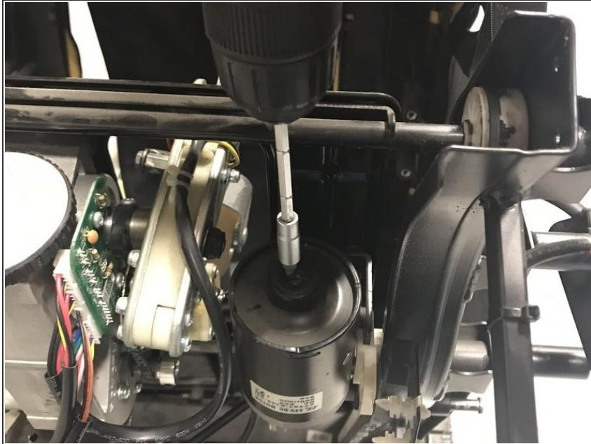
ⓘ Next attach a flat head bit to a cordless drill and insert it into the top of the Up and Down motor. this will allow you to drive the mechanism out the top of the track.
