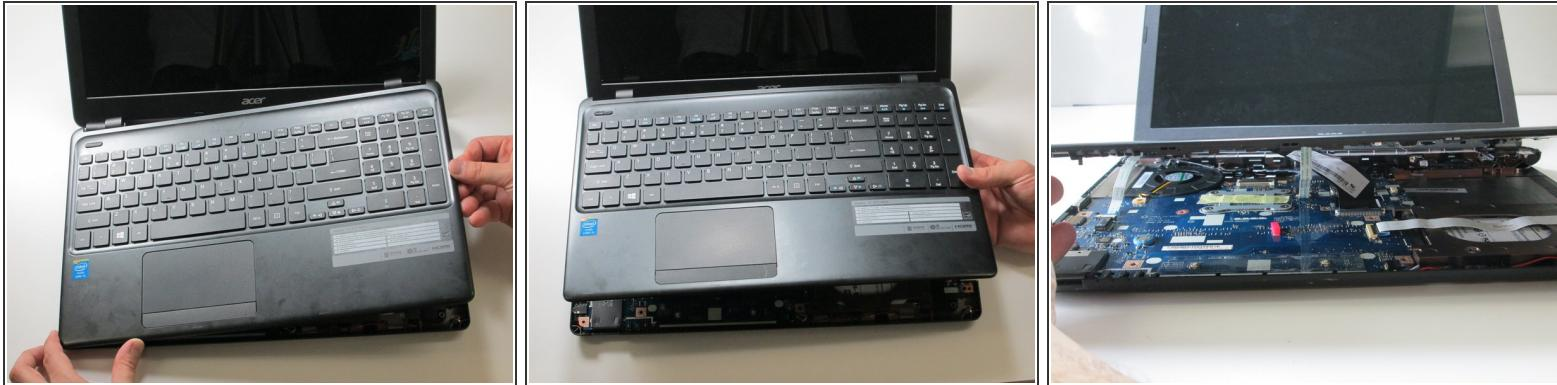
① Carefully detach the top panel of the laptop and slowly lift it up to reveal the internal components.
