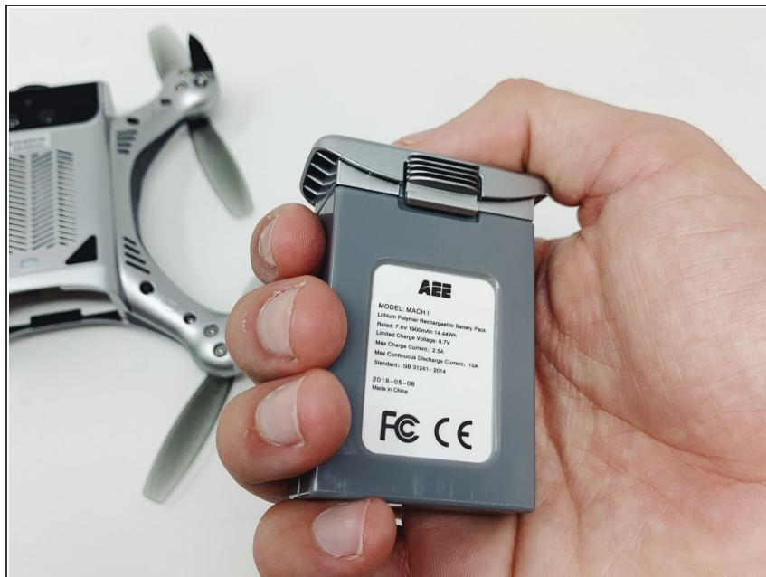
To replace the battery, simply slide it back into its place until the tabs click back into place. If you are having trouble doing this, you may be putting it in upside down. Try flipping it over and trying again.
