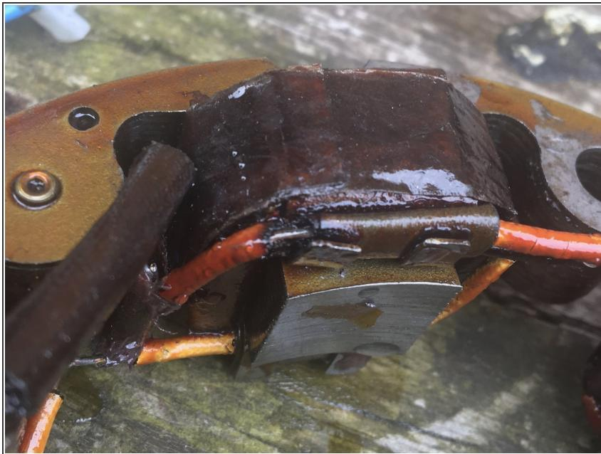
**i** The alternator stator is supposed to be insulated from earth.
