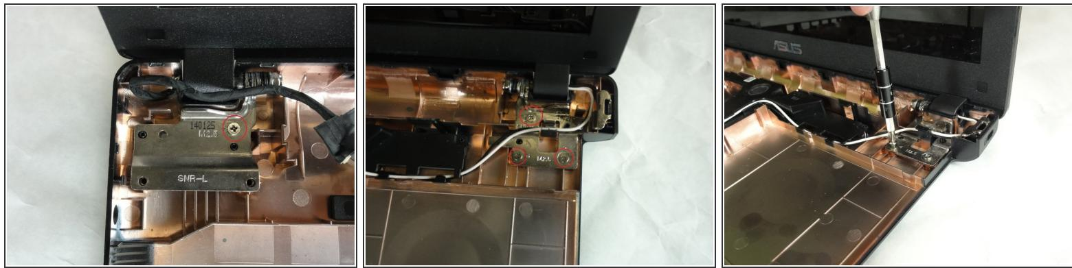
**⚠** Following these next steps will remove the Screen Module Anchors. Hold the screen in place as you follow these steps to prevent the screen from dropping.
