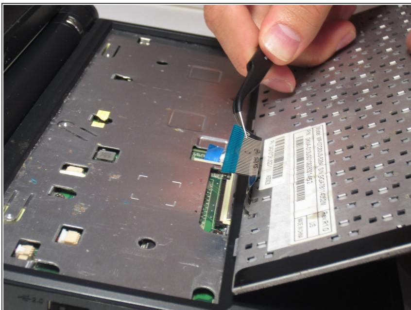
Carefully pull the cable out.
