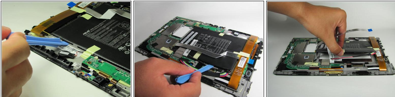
**(i)** Battery is glued to device. Remove with care.
