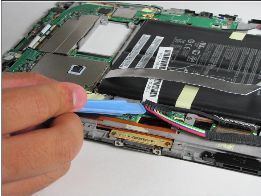
**⚠ Do NOT** pry the battery connector upward as shown in this photo. Instead, pull the connector straight out (in the direction of the wires).
